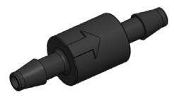
Lightweight Check Valve with inlets consisting of 1/8", 3/16" or 1/4" hose barbs. Outlet sizes include: 1/8", 3/16" or 1/4" hose barbs and 1/8" Male NPT. Valves are available without a spring or in 304 Stainless Steel or Hastelloy. The ball material consists of 316 Stainless Steel or Teflon. Body materials include: White Nylon, Polypropylene or Kynar. 125 psi maximum operating pressure and 140° F maximum operating temperature.
